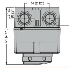
PG13.5 / M20 PG16 / M25 knockouts on top and bottom
