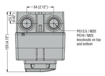
IEC/EN TYPE IP65 NON-METALLIC ENCLOSURE SWITCH DISCONNECTOR, THREE-POLE. WITH ROTATING BLACK HANDLE, 16A
