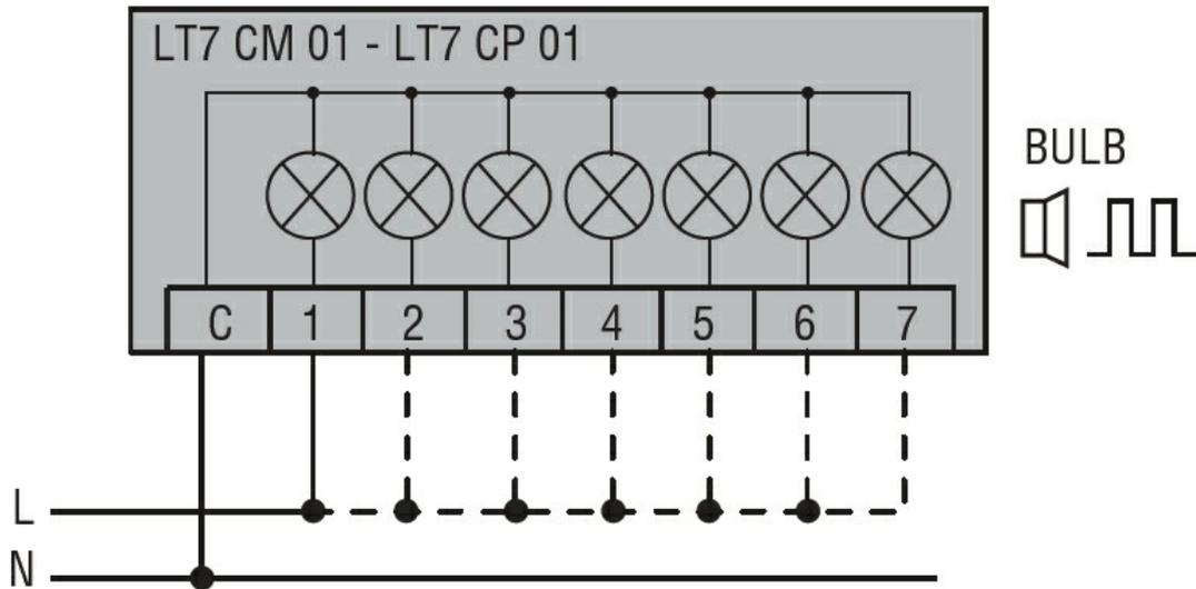
Connect terminals C and 1 as indicated to power the first module.
