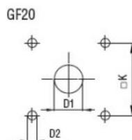
Drillings for 4 screws fixing (4V version).
