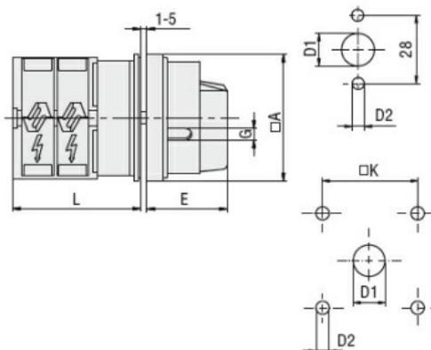
Standard drillings for 7GN125. Drillings on request for 4 screws fixing (4V version).
