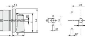
Standard drillings for 7GN125. Drillings on request for 4 screws fixing (4V version).
