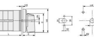
Standard drillings for 7GN125. Drillings on request for 4 screws fixing (4V version).
