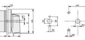
Standard drillings for 7GN125. Drillings on request for 4 screws fixing (4V version).
