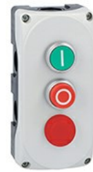
Grey control station LPZP3A8 complete with green flush pushbutton "i" LPCB1113 1NO, red extended pushbutton "o" LPCB2104 1NC and red pilot light 24V LPZP3B8901
