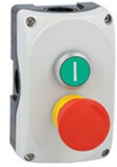
Grey control station LPZP2A8 complete with green flush pushbutton "I" LPCB1133 1NO and mushroom pushbutton turn-to-release LPCB6644 1NC LPZP2B8904
