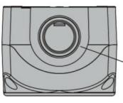
Knockout for M20/M25/PG13.5/PG16 (on top and bottom)
