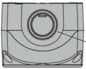
Knockout for M20/M25/PG13.5/PG16 (on top and bottom)
