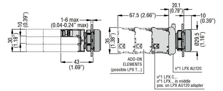
LED INTEGRATED LAMP-HOLDER, STEADY LIGHT Ø22MM PLATINUM SERIES, SCREW TERMINATION, 185...265VAC. GREEN
