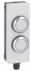
Control station for 40mm profile rails with two white flush illuminated pushbuttons, spring return, 5...35VAC/DC, 1NO each LP4P2B8901
