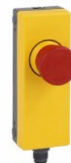
Control station for 40mm profile rails with mushroom head pushbutton, latch, turn to release for emergency stopping, 2NC LP4P1B5600
