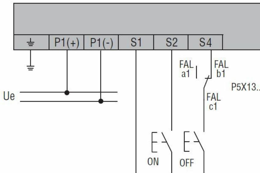
**Note:** Connect an NC contact of an alarm switch contact block in series with S4 to prevent remote closing of the MCCB after tripping due to overcurrent or short circuit.
