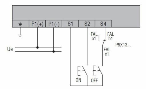
Note: Connect an NC contact of an alarm switch contact block in series with S4 to prevent remote closing of the MCCB after tripping due to overcurrent or short circuit.
