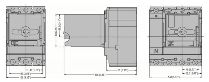
electric MOTOR OPERATOR FOR REMOTE OPERATION FOR P5ME...100/160/250, 230VAC / 220VDC
