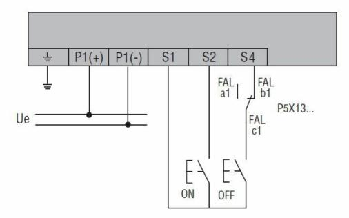
**Note:** Connect an NC contact of an alarm switch contact block in series with S4 to prevent remote closing of the MCCB after tripping due to overcurrent or short circuit.
