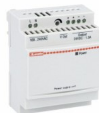
Zasilacz 100... 240 VAC/24VDC; 1,3A LRX1V3D024
