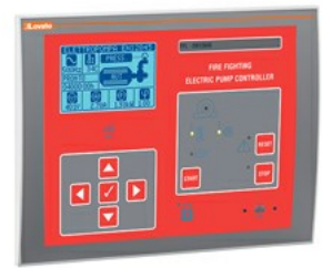
Electric fire pump controller, supply 24VAC or 100-240VAC, built-in RS485, expandable with EXP.. Modules FFL...EP
