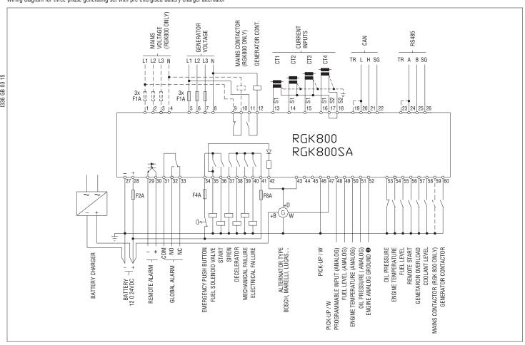
• Reference earth/ground for analog sensors to be connected directly on the engine block.
