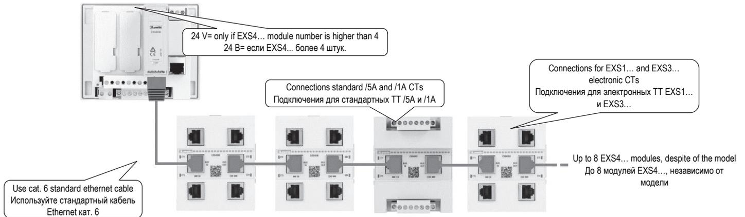
MECHANICAL DIMENSIONS, TERMINAL POSITION AND WIRING DIAGRAMS
