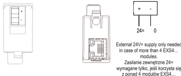
External 24V= supply only needed in case of more than 4 EXS4... modules.
