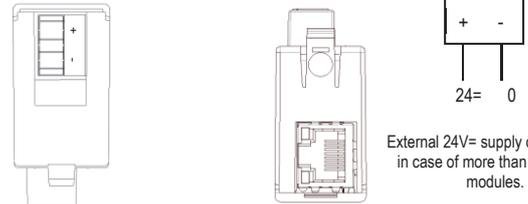
External 24V= supply only needed in case of more than 4 EXS4... modules.
