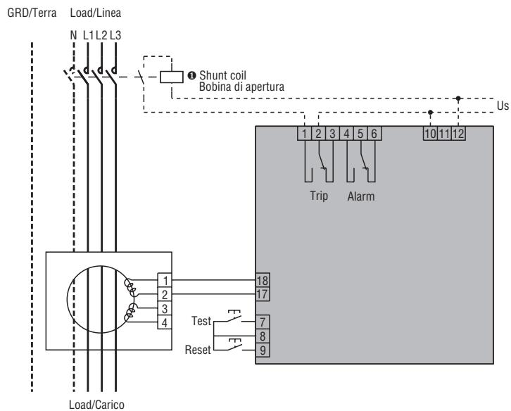
● The coil connection can vary depending on the connected type of device (contactor, breaker with shunt trip release or breaker with undervoltage trip release).
