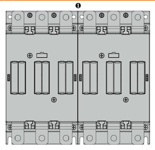
The BFX5500 interlock is mounted inside the 2 contactors without dimesions increasing.
