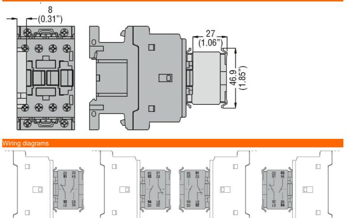
The termination of the G218 auxiliary contact has more than one numbering due to the fact that the block can assume various mounting positions. See the numbering in boldface for a correct interpretation.
