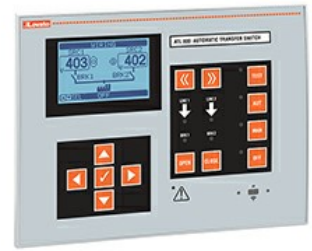
Automatic transfer switch controller for 2 power sources and one tie-breaker, three phase control, with LCD display, built-in RS485, expandable ATL800
